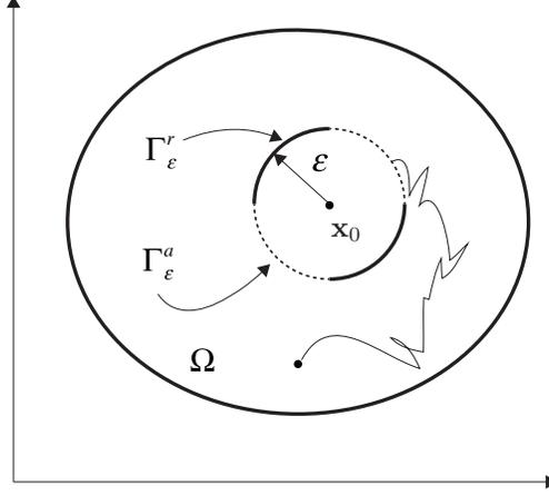
Figure 1: Schematic diagram of a bounded region  $\Omega$  with a trap composed of reflecting (solid lines) and absorbing (dashed lines) sections,  $\Gamma_\varepsilon^r$  and  $\Gamma_\varepsilon^a$ .
