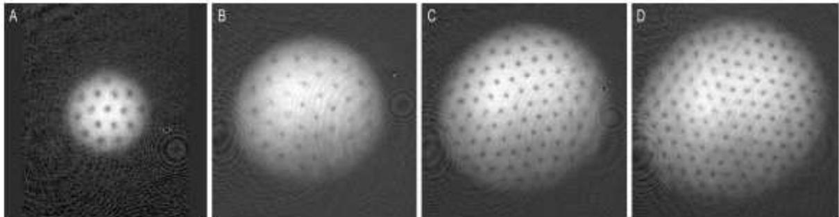
Slight asymmetries in the density distribution were due to absorption of the optical pumping light.
