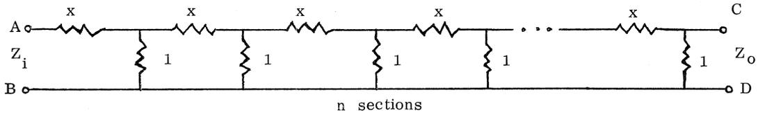
Assume that the terminals A and B are open. We desire the resistance as measured across terminals C and D. For  $n$  ladder sections, let us assume that the resistance is  $Z_n$ , and consider the output  $Z_o$ .
