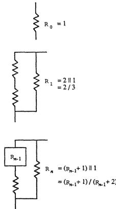
FIGURE 2. Source of the recurrence relation for resistance
