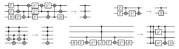
The bottom right circuit above is a relative phase Toffoli gate implementation taken from [6]. The utility of decompilation is apparant here, as both the fact that it implements a Toffoli up to phase and the exact form of the relative phase can be readily observed from the decompiled circuit.
