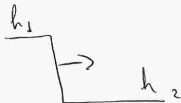
Where  $x_s = x_s(t)$  is the location of the bore which moves to the right in time
